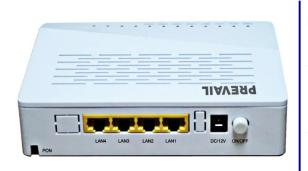
WXP4200-S series terminal products are mainly used for FTTH, FTTB, FTTC and other scenarios. They can be used for optical fiber to building network access, video monitoring, WIFI hot spot deployment and other applications. Based on 10G-XPON technology, 10 Gigabit of uplink bandwidth is provided for users to meet ultra-high bandwidth business needs.
